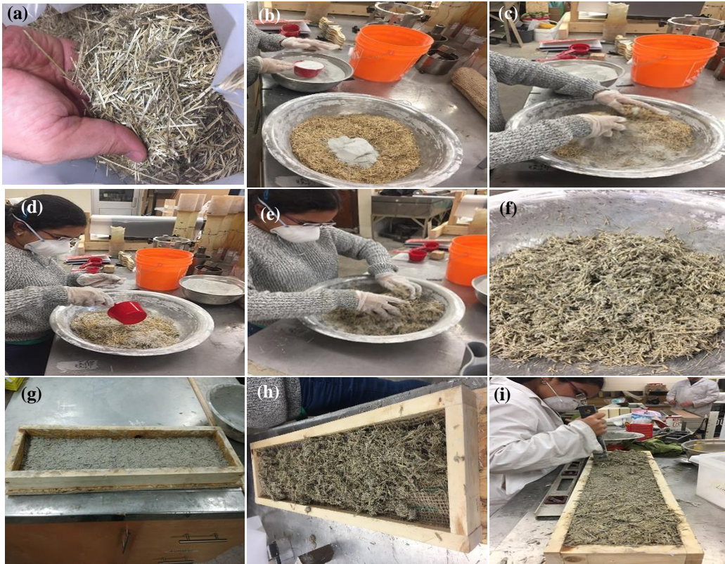
Figure 2. Specimen preparation: (a) flax shives; (b) adding binder to flax shives; (c) mixing binder with flax shives; (d) adding water to mix; (e) mixing water with flax and binder; (f) flax-lime mix ready to be used; (g) formwork filled and compacted to half; (h) jute fabric placed and next flax-lime layer cast; and (i) the last layer compacted.
